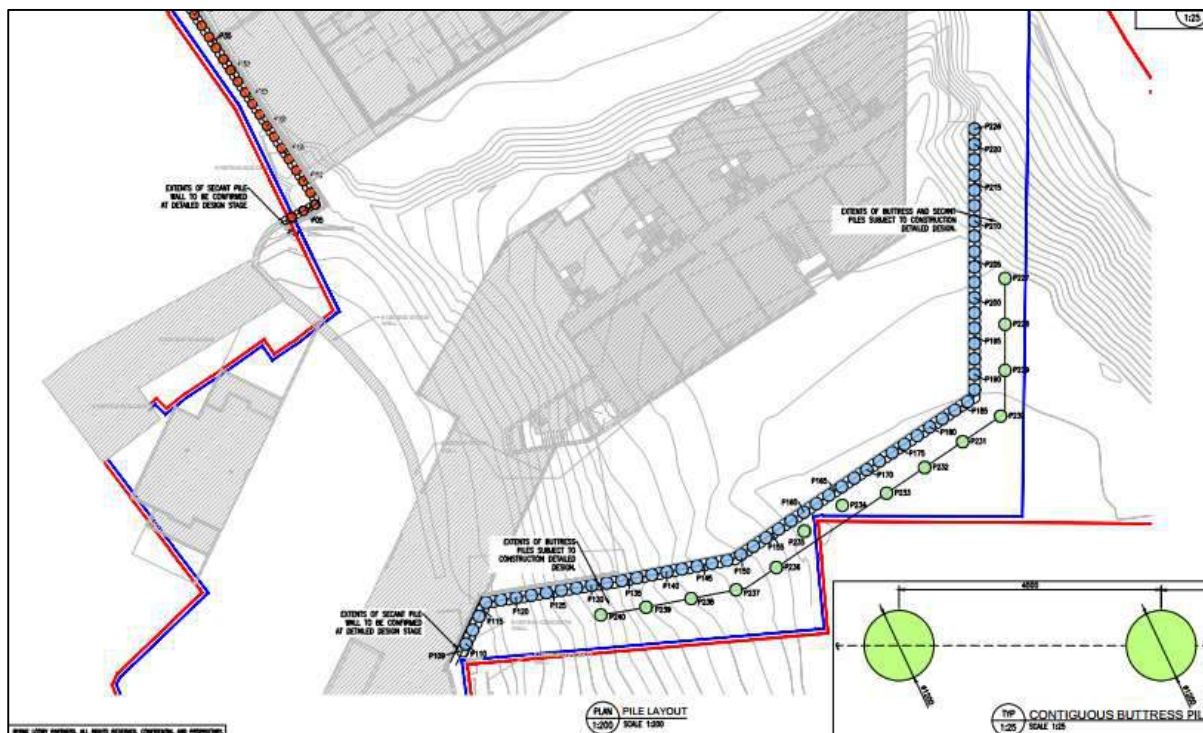
Figure 5.2: Proposed Secant Pile Wall Layout
