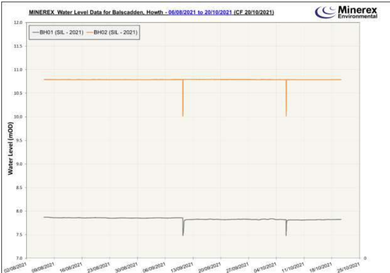
Figure 4.2 Continuous water level data from BH01 and BH02.
